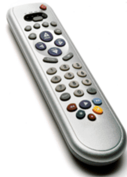
Remote controls for TV/VCR
